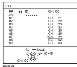
**3 Press the ▼/▲ buttons to choose "CC" or "CH" according to the CH/CC number of the TV channel**
