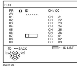
**3 Enter a channel name (ID). Press the ▼/▲ buttons to choose a character. Press the ◀/▶ buttons to move the cursor.**
