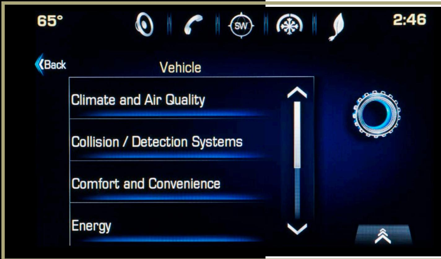
Some vehicle features can be customized using the controls on the infotainment system. The Vehicle Settings menu may include Climate and Air Quality; Collision/Detection Systems; Comfort and Convenience; Energy; Lighting; Power Door Locks; and Remote Lock, Unlock, Start.
