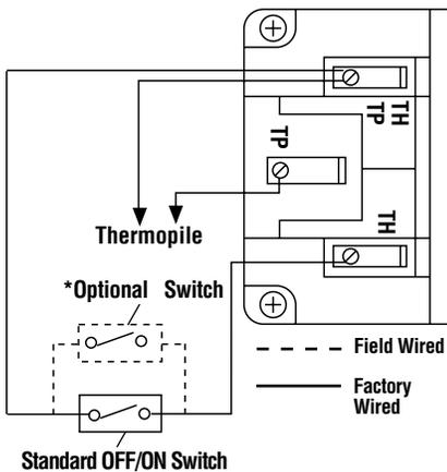
\* Optional Kits Installed - OFF/ON wall switch, wall thermostat or remote control receiver. Note: Turn the appliance-mounted OFF/ON burner control switch to the OFF position if any of these kits are installed.
