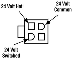
Check For Damaged or Missing Terminals in Connector
