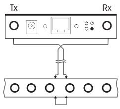
If the fiber optic cables are unbroken, the fiber link LED will illuminate green. As before, note that the fiber test mode LED will be red, and the Power LED will be green.
