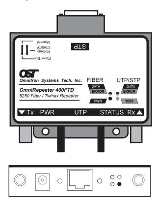
The meaning of the LEDs is shown on the cover of the OmniRepeater 400FTD and in the tables below.
