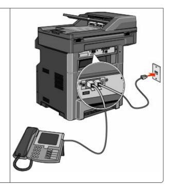
Telephone or a telephone with an integrated answering machine
