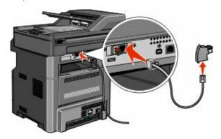
**3** Connect the adapter into the N slot of an active analog telephone wall jack.
