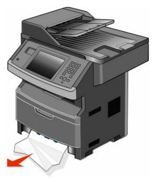
If you do not see the jam, open the front door, and then remove the photoconductor kit and toner cartridge.
