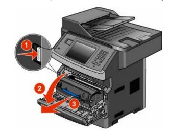
**2** Lift the flap at the front of the printer, and then remove any jams.
