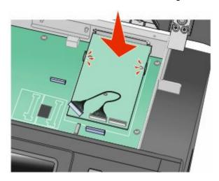
Insert the long thumbscrew, into the hole closest to the white connector, and turn it clockwise enough to hold the ISP in place. Do not tighten the thumbscrew at this time.
