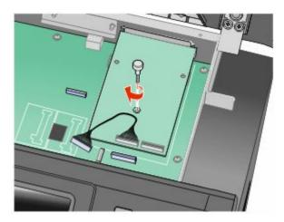
Attach the two provided screws to secure the ISP mounting bracket to the system board cage.
