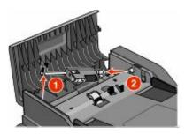
**4** Use a clean, lint-free cloth dampened with water to wipe the separator rollers.
