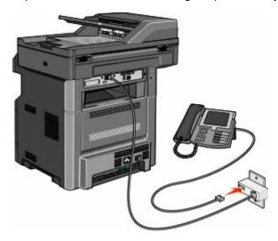
**3** Remove the protective plug from the printer EXT port **1**.
