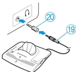
**i** With most TVs, the headphone socket is located at the front or sides.
