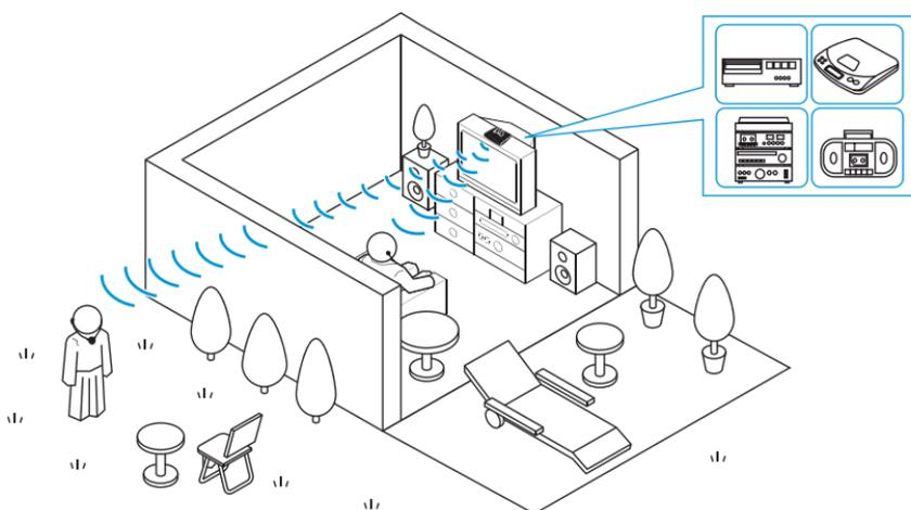
When the stethoset receiver leaves the range of the transmitter, it produces warning signals and then automatically switches off after 3 minutes.
