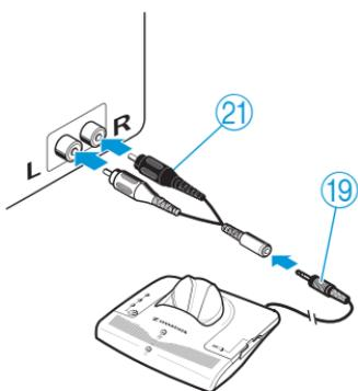
**i** With most TVs, the RCA socket is located at the rear. If your TV has several RCA sockets, use the socket **RCA output**.
