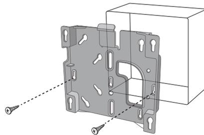
Securing the antenna to the mounting plate
