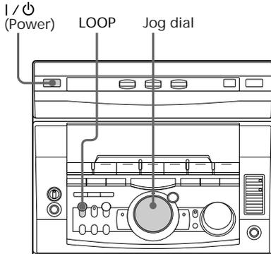
➔ Press and hold LOOP during playback at the point you want to start the Loop function, and release to resume normal play.
