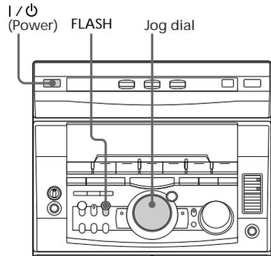
➔ Press and hold FLASH during playback at the point you want to start the Flash function, and release to resume normal play.
