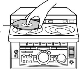
To insert a third disc, press DISC SKIP/EX-CHANGE to rotate the disc tray.
