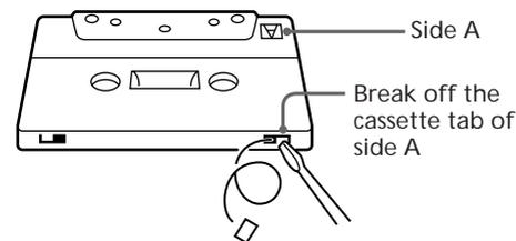
If you later want to reuse the tape for recording, cover the broken tab with adhesive tape. However, be careful not to cover the detector slots which allow the tape player to automatically detect the type of tape.
