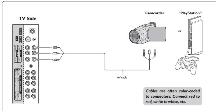
Connect the Audio/Video cables between the Audio (L/R)/Video jacks on the unit and camcorder.
