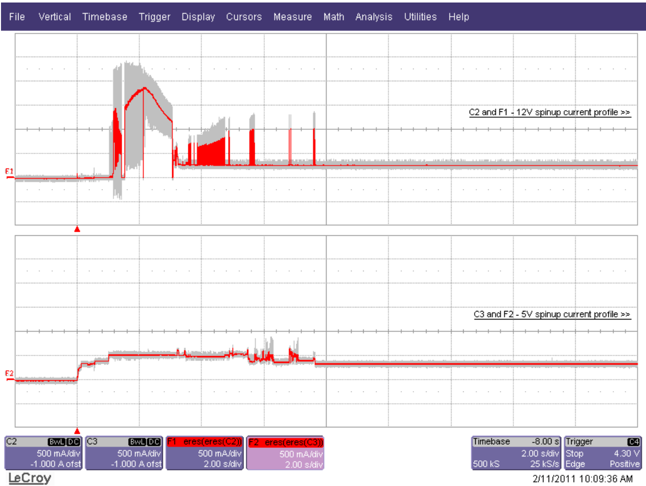
Figure 3. 500GB model current profiles
