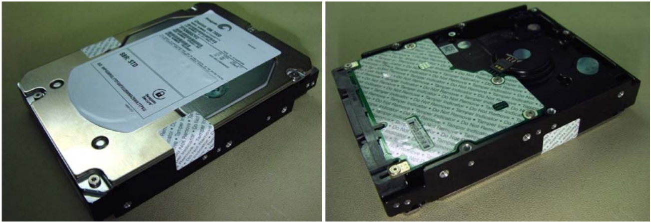
Figure 13. Example of FIPS tamper evidence labels.
