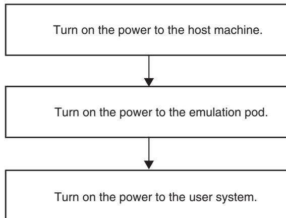
To turn on the power of the emulation pod, press the power switch on the rear of the 2140 main unit toward the "I" side.
