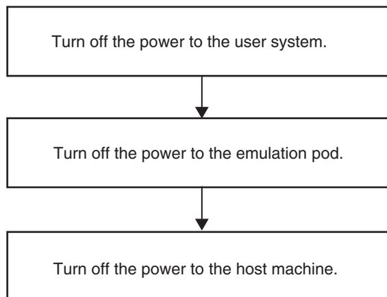
To turn off the power of the emulation pod, press the power switch on the rear of the 2140 main unit toward the "0" side.
