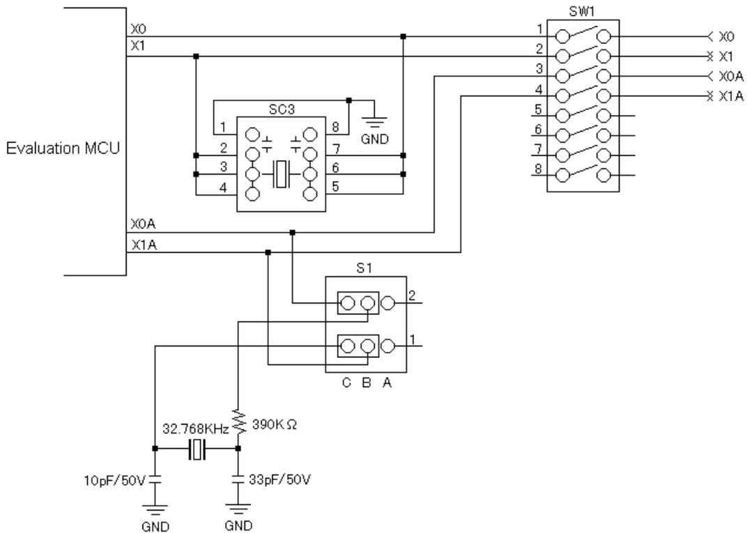
Figure 2.6-2 Crystal mounting example
