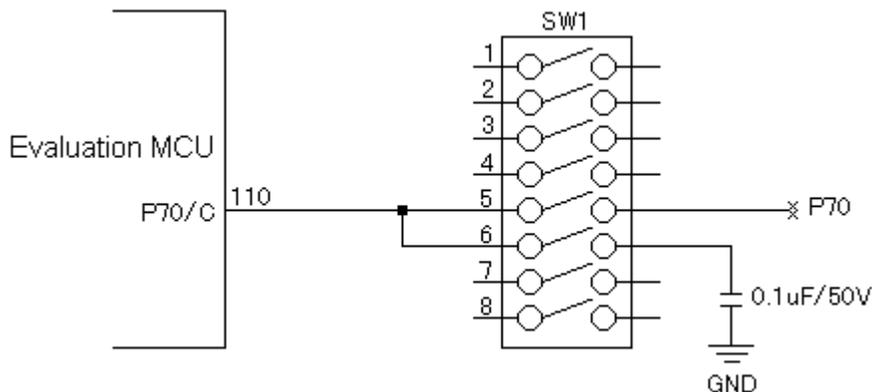
**Table 2.8-1 Jumper switch for setting the C-pin circuit connection**
