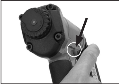
Figure 7. Trigger switch, bump fire mode.
