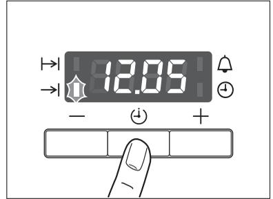
2. Using the  $+$  or  $-$  button, set the required switch-off time.
