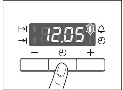
2. Using the + or - button, set the required Countdown (max. 2 hours 30 minutes).
