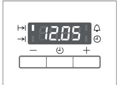
When the time has elapsed, the function indicator will flash, an acoustic signal will sound for 2 minutes and the oven will switch itself off.
