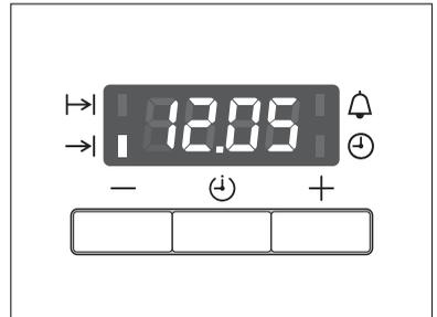
When the time has lapsed, the function indicator will flash, an acoustic signal will sound for 2 minutes and the oven will switch itself off.
