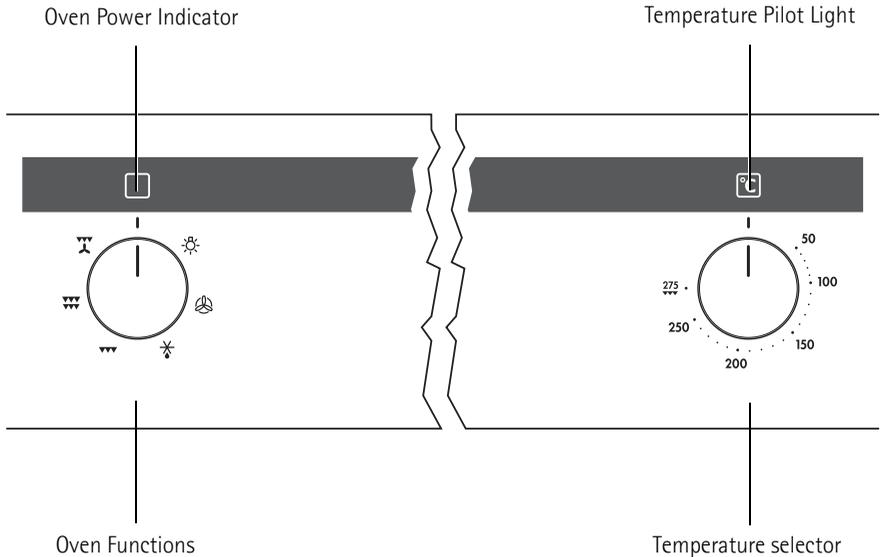
1. Turn the oven functions control knob to the desired function.
