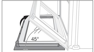
4. Take hold of the door trim (B) on the upper edge of the door at both sides and press inwards to release the clip seal. Then remove the door trim by pulling it upwards.
