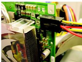
After installing the GV-3D1-7950-RH to your computer, please remember to connect at least one power cable on the graphics card to the power supply connector. We suggest you to connect both of the two power cables on the graphics card to the power supply to achieve optimal graphics performance.
