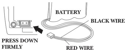
**NOTE:** It is important to maintain the polarity (black and red wires) to the jack inside the compartment as shown in the illustration.
