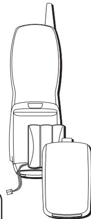
**NOTE:** If the battery is not properly installed in the handset, or if the battery pack is not properly connected to the jack inside the battery compartment, “*NO BATTERY*” shows in display when the handset is placed in the base cradle.
