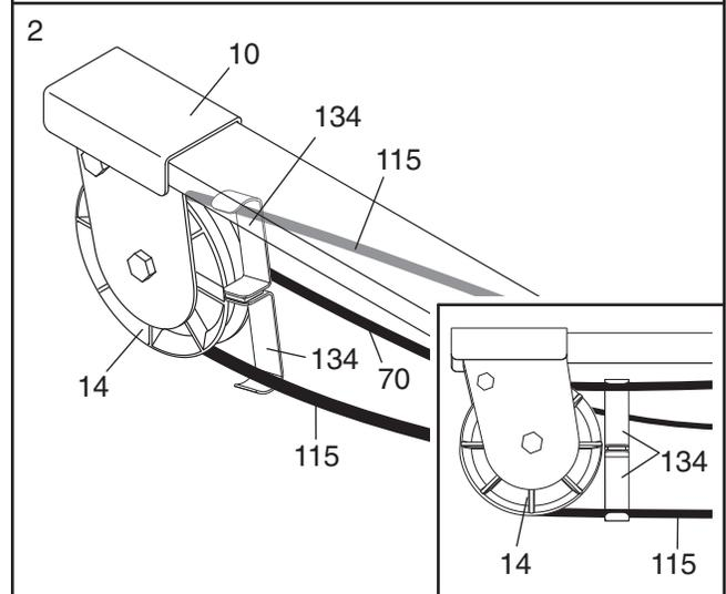
3. Locate the 3/8" x 38mm Tension Screw (59) on each end of the Resistance Bar (9). Alternately tighten each Screw one turn at a time until the two Tension Gauges (134) are pulled apart by the Upper Cable (115).
