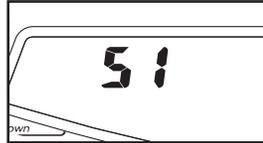
The right display will show the total number of miles (or kilometers) that the walking belt has moved. In addition, the right display will show the letter "E" for English miles or the letter "M" for metric kilometers. Press the Speed increase button to change the unit of measurement if desired.
