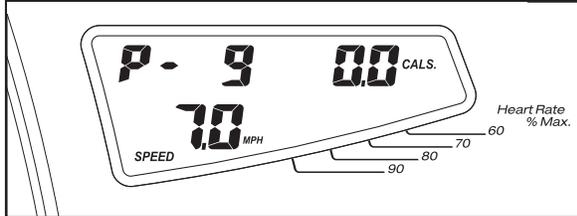
If the custom program has not yet been defined, three columns of indicators will scroll across the matrix in the left display. **If more than three columns of indicators appear, see HOW TO USE A CUSTOM PROGRAM on page 16.**
