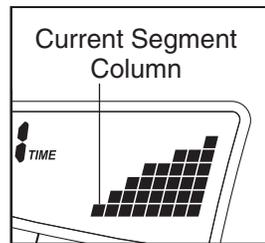
When the first segment ends, *all target heart rate settings will move one column to the left.* The target heart rate setting for the second segment will then be shown in the flashing Current Segment column.
