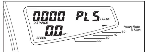
**If heart rate program 8 is selected,** the letters “PLS” and the maximum target heart rate setting for the program will begin to flash in the right display. If desired, change the maximum target heart rate setting by pressing the + or – button beside the Enter button (**see EXERCISE INTENSITY on page 24**). Then, press the Enter button. Note: If the maximum target heart rate setting is changed, the intensity level of the entire program will change.
