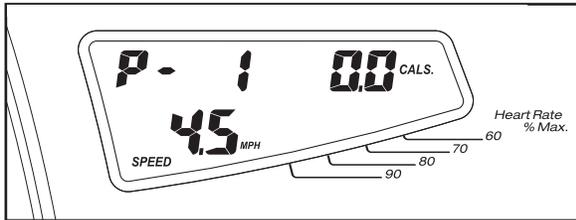
When a preset program is selected, the left display will flash the maximum incline setting of the program for a few seconds, and the right display will flash the maximum speed setting. The left display will then show how long the program will last. In addition, a profile of the speed settings of the program will scroll across the matrix in the left display.
