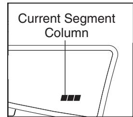
When the first segment of the program ends, the current speed setting and the current incline setting will be stored in memory. *The three columns of indicators will then move one column to the left, and the speed setting for the second segment will be shown in the flashing Current Segment column.* Program a speed setting and an incline setting for the second segment as described above.
