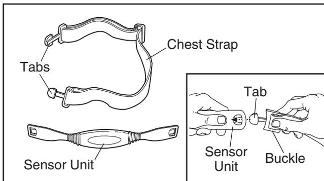
Insert the tab on one end of the chest strap into the hole in one end of the sensor unit, as shown in the inset drawing above. Press the end of the sensor unit under the buckle on the chest strap. The tab should be flush with the front of the sensor unit.
