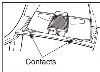
To use the handgrip pulse sensor, **stand on the foot rails** and hold the handgrip pulse sensor with your palms resting on the metal contacts; **avoid moving your hands**. When your pulse is detected, the heart-shaped indicator in the right display will flash each time your heart beats, one or two dashes (– –) will appear, and then your heart rate will be shown. **For the most accurate heart rate reading, continue to hold the contacts for about 15 seconds.**
