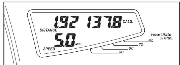
The right display will also show your heart rate when you use the handgrip pulse sensor or the chest pulse sensor. In addition, during heart rate programs the right display will show a heart rate bar that shows your heart rate as a percentage of your estimated maximum heart rate (see step 3 on page 17 for an explanation of your estimated maximum heart rate). For example, if four to six segments of the bar appear, your heart rate is between 60% and 70% of your estimated maximum heart rate.
