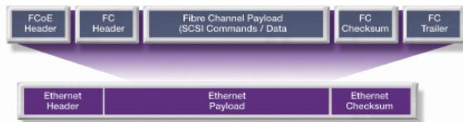
Figure 2 FCoE encapsulation in Ethernet
