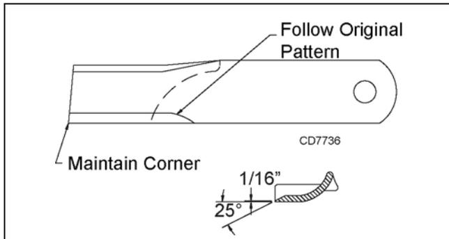
Figure 14. Blade Sharpening
