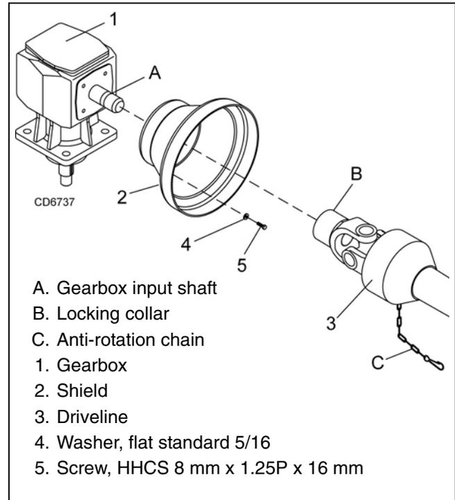
Figure 30. Driveshaft Installation
