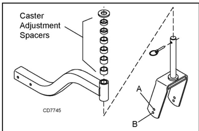
**Figure 6.** Height Adjustment with Caster Arm Spacers
