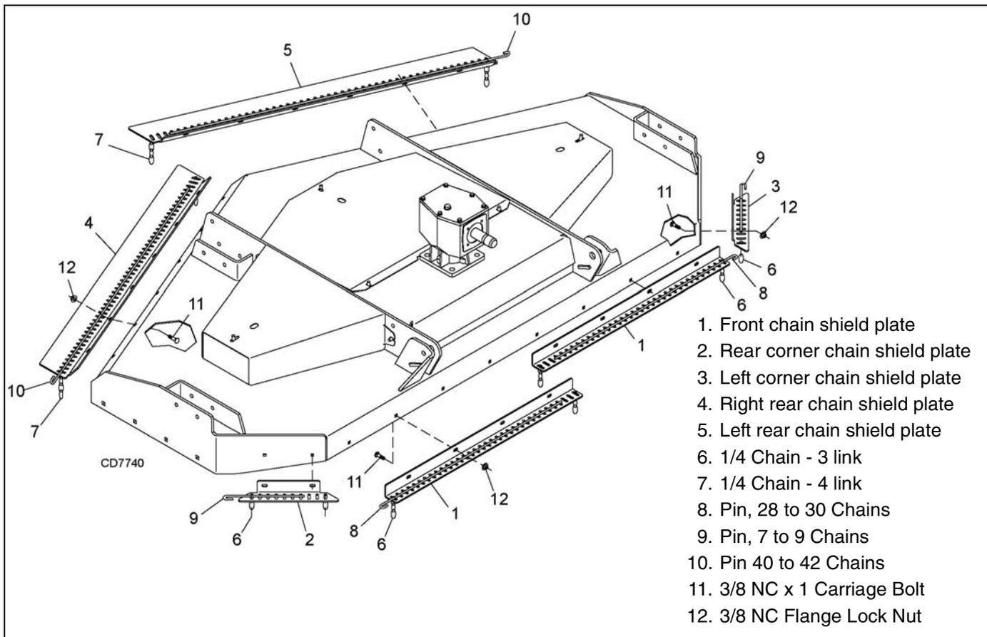
Figure 31. Chain Shield Installation
