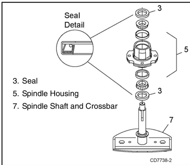
**Figure 16.** Spindle Disassembly
