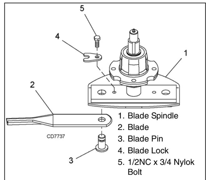
Figure 12. Blade Removal
