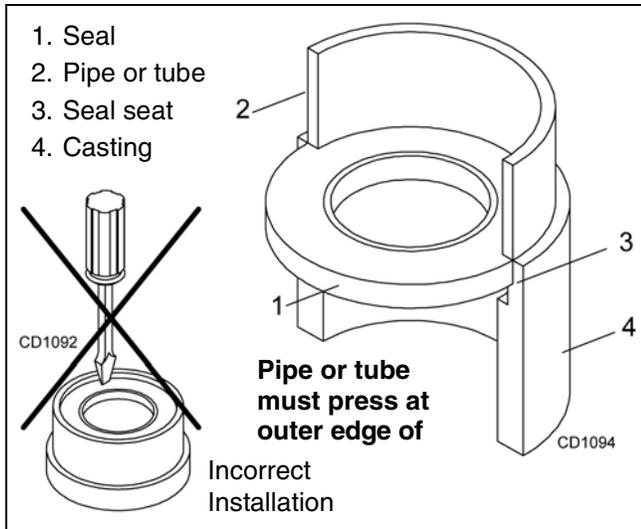
**Figure 19.** Seal Installation
