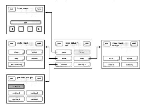
The **name** button provides a way to customize the names of the inputs as displayed on the input selection screens. For example, you might want to name an input "CDP-100" for the Classé CD player you might have connected there. To do so, use the four buttons along the bottom of the Input Name menu to change the default name of any given input to something more specific to your system, as follows:
