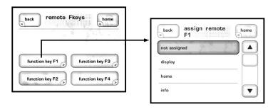
The remote control supplied with the SSP-600 has four **function** keys (**Fkeys**) that allow you to have instant, easy access to specific system functions that might otherwise be buried in a menu somewhere.
