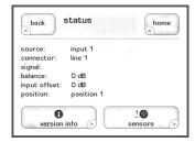
The **status** screen provides several items of information about the current operation status of the SSP-600, as well as access to information on the software used in and the internal sensors of the SSP-600.
