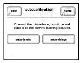
Simply plug in the microphone to the **mic** input on the rear panel, place the microphone at the desired position, and then press **auto levels** and **auto delays** in turn, allowing the SSP-600 to run its tests and establish the correct settings for you.
