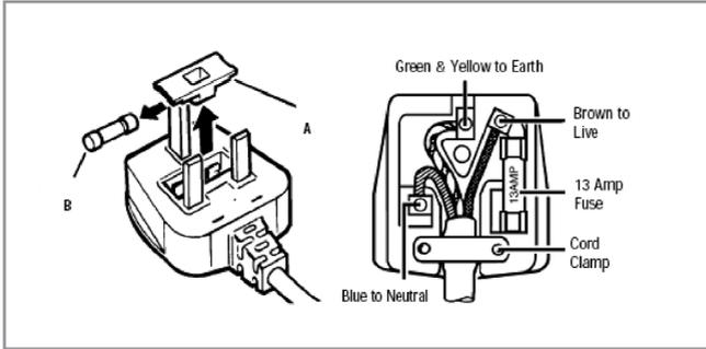
The mains lead of this appliance has been fitted with a BS 1363A 13 amp fused plug. To change a fuse in this type of plug, follow the steps below:
