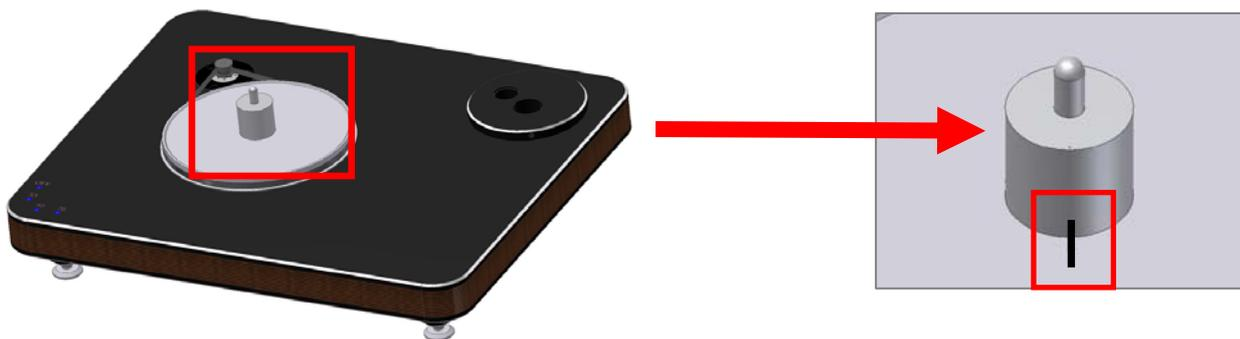
**Pic. 6:** Alignment of sub-platter and bearing markings
