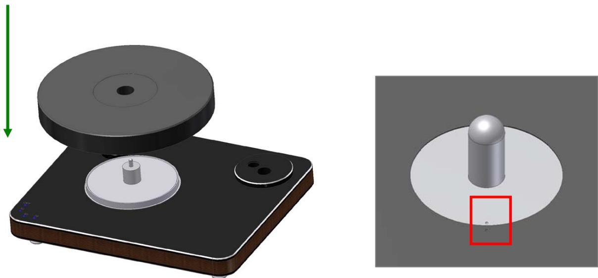
**Pic. 7:** Seating the platter on to the bearing
