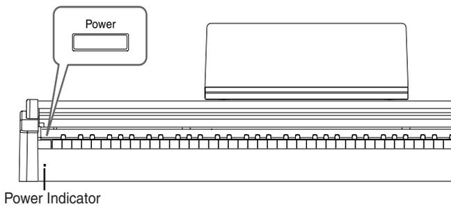
To turn the power off, turn the [VOLUME] knob all the way to the left, and press the [Power] switch.
