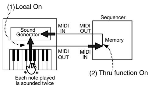
Local Control ON: The keyboard and the internal sound generator are in a linked state.
