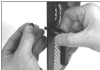
**6c.** Slip latch bar onto handle threads. Align "D" slot in latch bar with flat on handle threads. The latch bar should point toward the left. Assemble the second hex nut to finish the assembly. This hex nut functions as a "jam nut", and will tighten against the first hex nut assembled in Step 5b.
