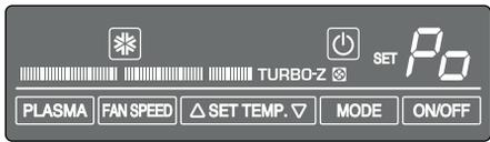
3 To cancel the **TURBO-Z** mode, press the **TURBO-Z** button again or the Auto Swing Direction Control Button (Up & Down, Left & Right) or Operation Mode Button and the unit will operate in High. Fan speed on cooling mode.
