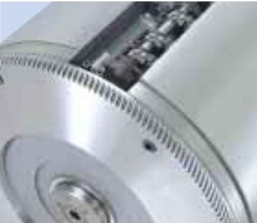
Ultra-high-precision helical gears are used on the impression cylinder
