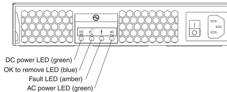
Figure 34. Power-supply LEDs
