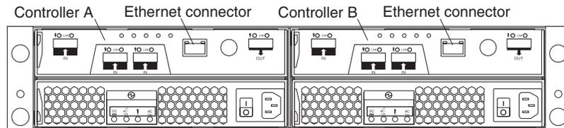
Figure 23. Ethernet port locations on a dual-controller DS3200
