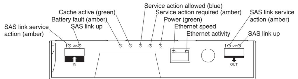
Figure 36. Controller LEDs
