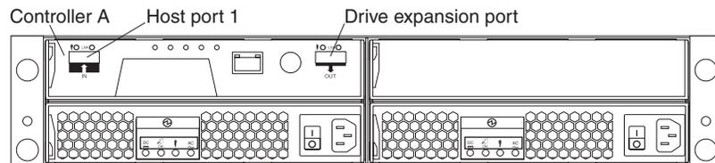
Figure 13. Single-controller DS3200 storage subsystem ports and controller
