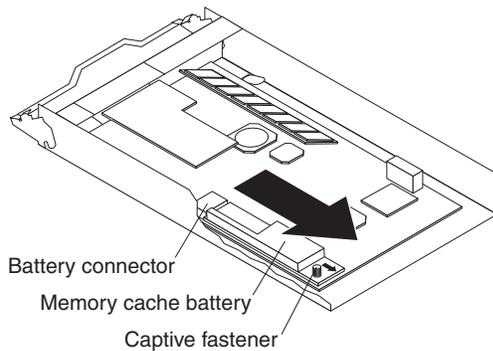
Figure 41. Removing the battery unit from the controller
