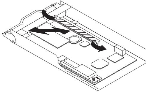
Figure 54. Removing the DIMM from the controller
