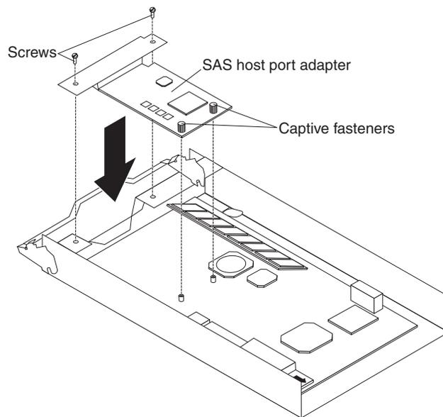
Figure 44. Installing a SAS host port adapter
