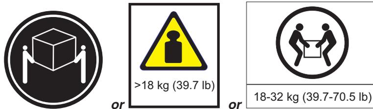
**The weight of this part or unit is between 18 and 32 kg (39.7 and 70.5 lb). It takes two persons to safely lift this part or unit. (C009)**
