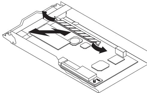
Figure 55. Installing the DIMM in the controller
