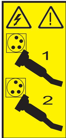
**Attention:** Turning off and turning on power without waiting for the storage subsystem disk drives to spin down can damage the drives and might cause data loss. Always wait at least 70 seconds after you turn off the power before you turn on the power again.
