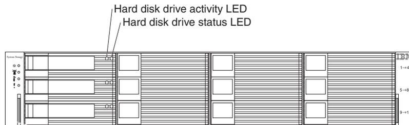
Figure 45. Hard disk drive LEDs
