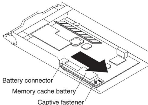
Figure 50. Removing a battery unit from the controller
