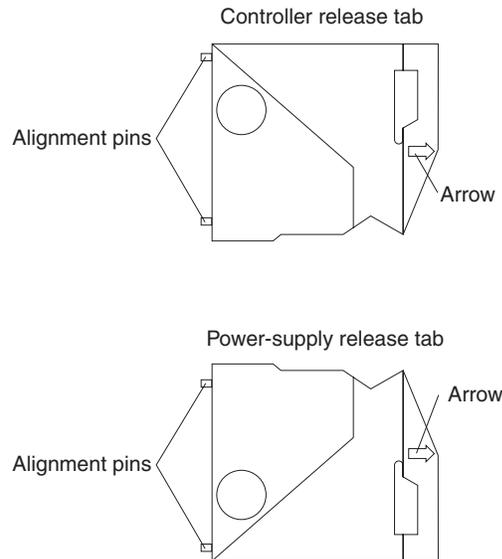
Figure 58. Controller and power supply release tabs
