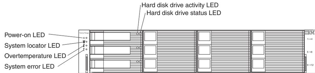
Figure 35. Front LEDs and controls
