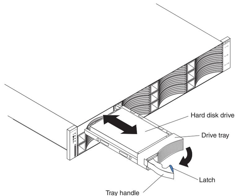
Figure 47. Installing and removing a hard disk drive
