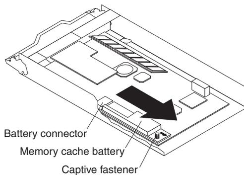
Figure 53. Removing the battery from the controller
