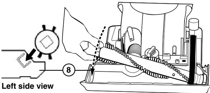
9. Align left end cap with square in base. Push end cap into place; see left side view.
