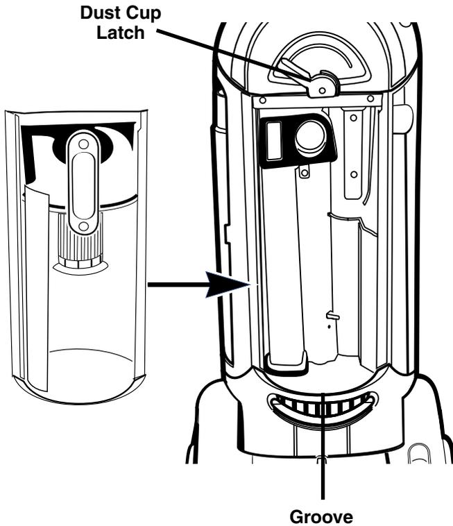
4. Replace dust cup by aligning front of the bottom of dust cup into groove on cleaner. Pivot dust cup up against cleaner and rotate the dust cup latch to the right to secure.
