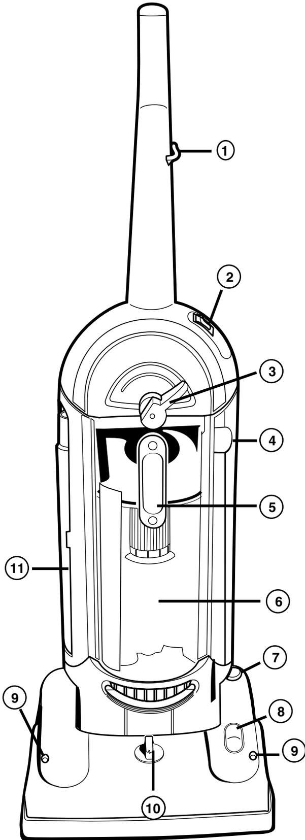
1. **Cord Retainer.** To use, push electrical cord down into cord retainer.
