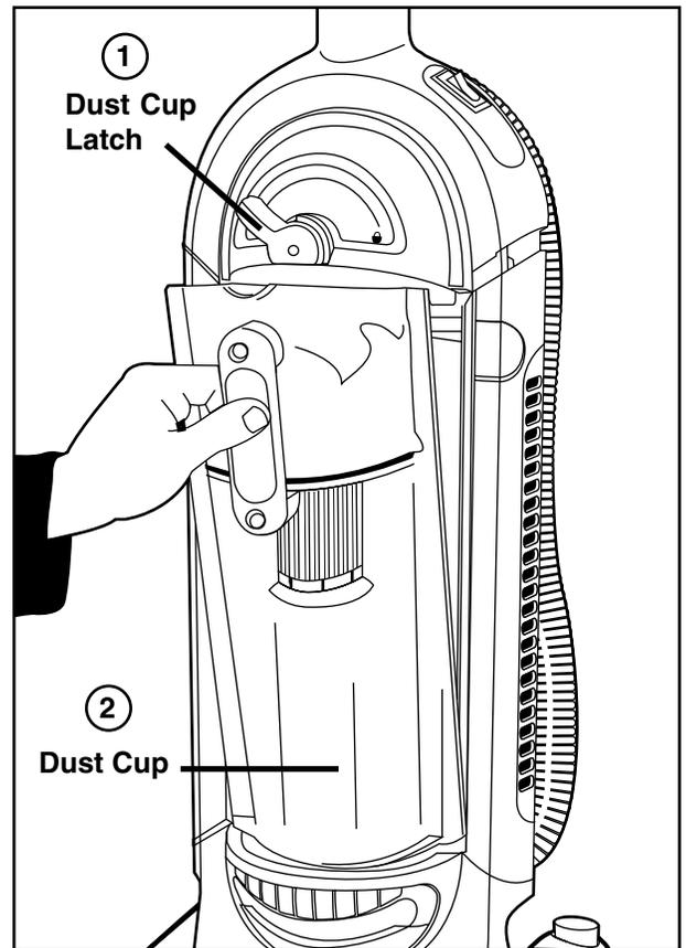
Release dust cup by rotating dust cup latch to the left pointing to the unlock symbol (🔓). Pivot dust cup out and away from cleaner and remove.
