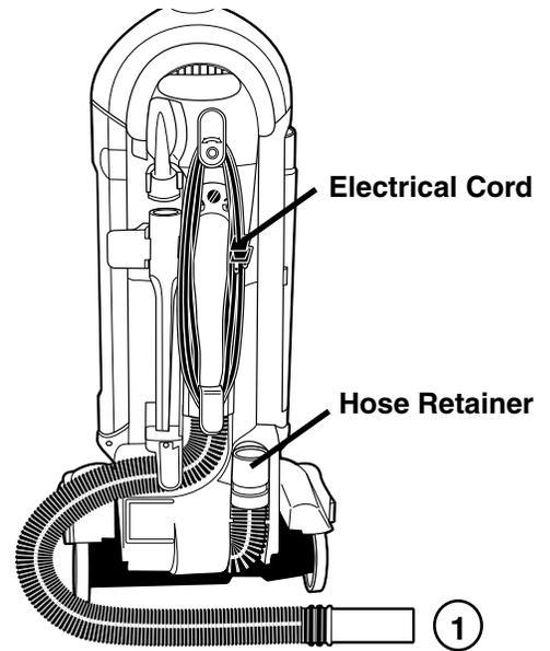
1. Remove hose from hose retainer and check suction at end of hose.
