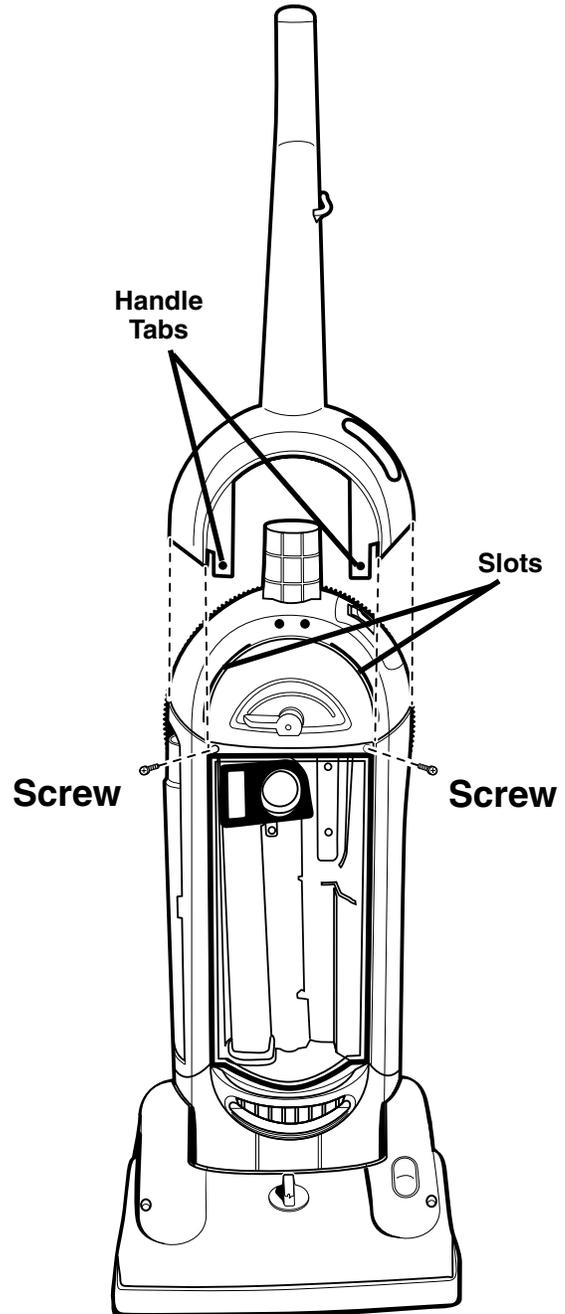
2. Position handle as above. Slide the handle down over the top of the unit, inserting handle tabs into slots on unit.
