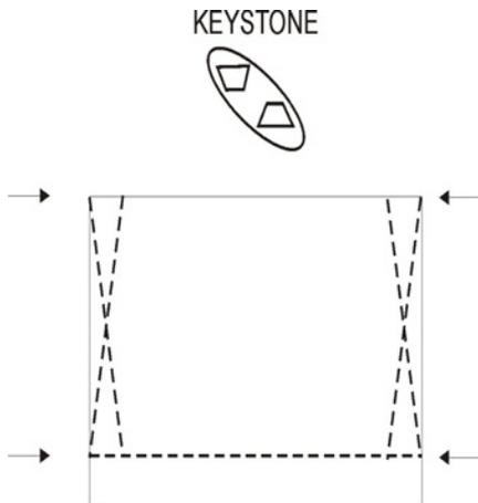
To adjust image vertically and make a square image. Adjust the keystone function by pressing the keystone button on the remote control or through OSD menus.
