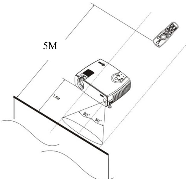
Users, using the remote control can, either point it directly at the IR Transceiver, or stand behind the unit and point it at the projected image.
