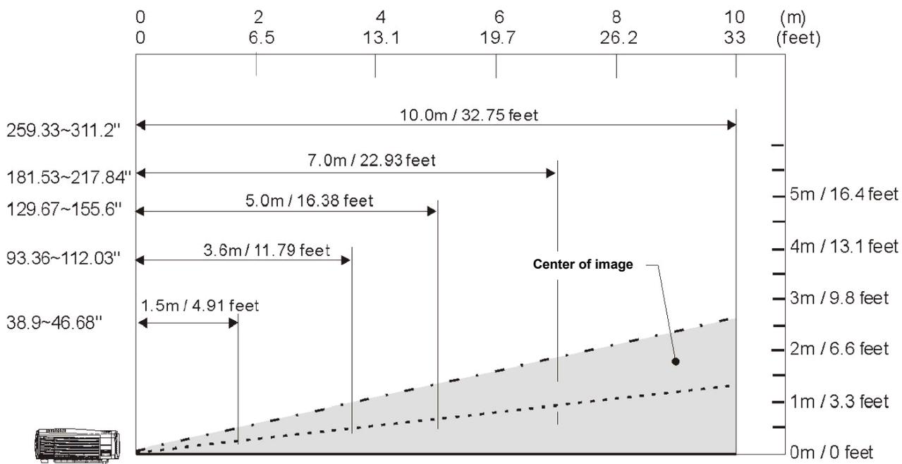
Figure 1 : Projection Distance vs. Image Size
