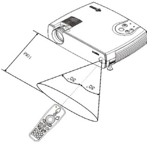
The projector is equipped with an IR Transceiver located at the front cover of the unit for the receipt of remote control transmission.
