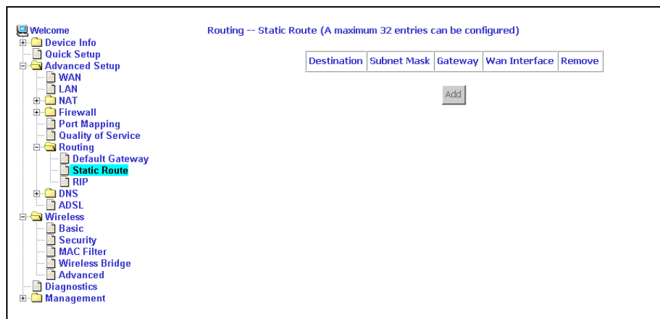
Figure 59: Static Route Setup
