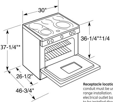
**Receptacle locations:** Locally approved flexible service cord or conduit must be used because terminals are not accessible after range installation. See shaded area in drawing for location of electrical outlet box. Recommended outlet locations allow range to be installed directly against wall.
