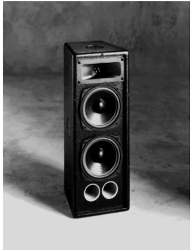
The ultra-compact, high-power reinforcement speaker system shall be a passive 3-way type with two 5-inch low-frequency loudspeakers, front mounted in a ducted brass-reflex hardwood plywood enclosure with a high-frequency piezo-electric driver mounted on a 2" x 5" horn. The enclosure shall be fitted with three  $\frac{3}{8}$ "-16 threaded mounting points, and shall operate with a separate Control Electronics Unit.
