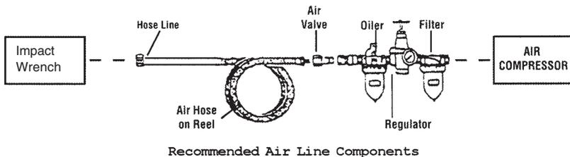
For best service you should incorporate an oiler, regulator, and inline filter, as shown in the diagram above. Hoses, couplers, oilers, regulators, and filters are all available at Harbor Freight Tools.
