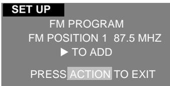
10. Press numeric keys 1 through 9 on the remote control to select the appropriate FM position.
