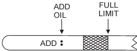
Figure 17. Engine Oil Dipstick
