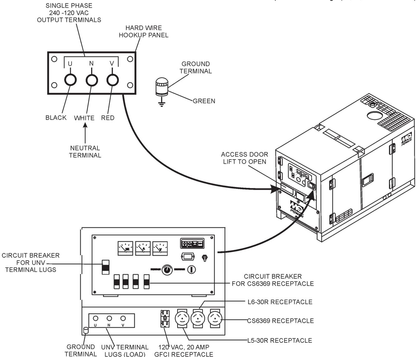
Figure 5. Output Terminal Panel
