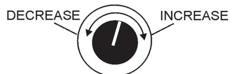
Figure 10. Voltage Regulator Control Knob
