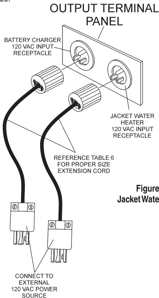
**Figure 36. Battery Charger & Jacket Water Heater Power Connections**
