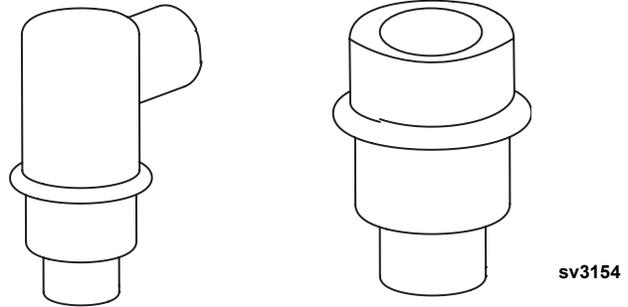
1. Remove check valve and tube assembly.
