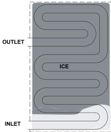
**Figure 7-4. Extremely Thin Ice Formation at Evaporator Inlet**
