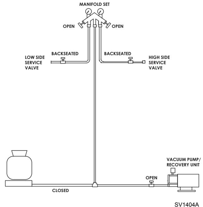
**Figure 7-7. Recovery/Evacuation Connections**
