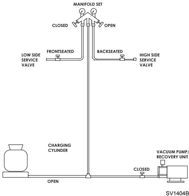
**Figure 7-8. Charging Connections**
