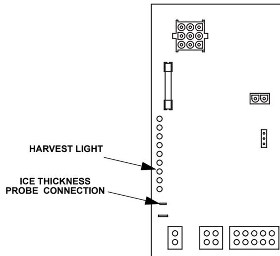
**Ice Machine Cycles Into Harvest Before Water Contact With The Ice Thickness Probe**
