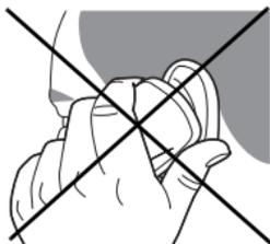
The antenna is integrated in your phone, under the back cover at the top.
