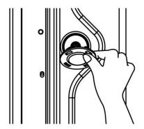
4. Adjust the level of washing machine by the adjustable feet. Please check if there is a gap between the four adjustable feet and the floor. If there is then adjust the level of the washing machine by turning the adjustable feet. Make sure that the machine does not sway and that it is completely level. After the adjustment is finished, turn the fixing nuts up tightly, so that the adjustment that has been made is fixed.
