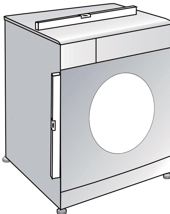
1. Loosen the lock nuts on the feet by hand.
