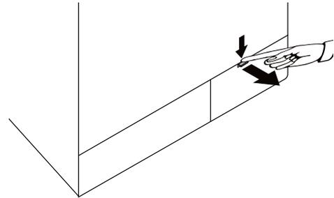
If the filter cap is one piece, pull the cap from both sides at the top to open.
