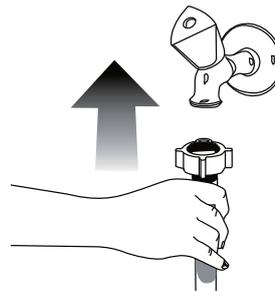
3. Open the taps completely after making the hose connection to check for water leaks at the connection points. If any leaks occur, turn off the tap and remove the nut. Retighten the nut carefully after checking the seal. To prevent water leakages and damages caused by them, keep the taps closed when the machine is not in use.
