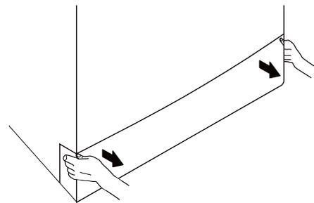
**i** You can remove the filter cover by slightly pushing downwards with a thin plastic tipped tool, through the gap above the filter cover. Do not use metal tipped tools to remove the cover.
