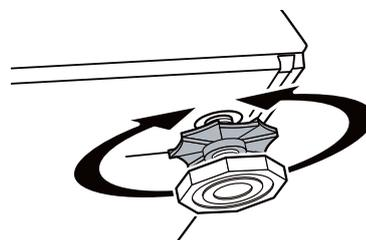
**!** Do not use any tools to loosen the lock nuts. Otherwise, they will get damaged.
