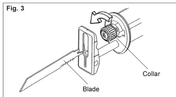
1. Depending on the job, the blade may be inserted with the teeth facing up or down. To install a blade, twist collar in the direction of the arrow while inserting the blade into the clamp until the tang butts against the collar.
