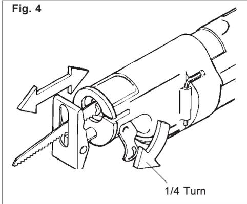
1. To adjust the shoe, pull the shoe release lever down 1/4 turn and slide the shoe forward or backward to the desired position.
