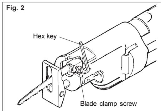
1. Depending on the job, the blade may be inserted with the teeth facing upward or downward.
