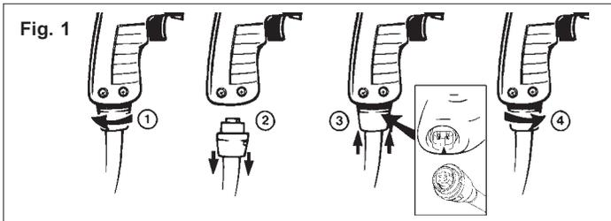
1. To remove the Quik-Lok® Cord, turn the cord nut 1/4 turn to the left and pull it out.
