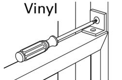
Attach the window locking brackets (one on each side) with Type C screws.
