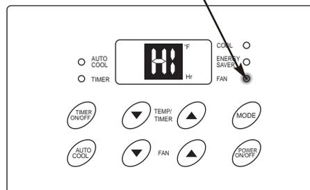
Note: Use this function only when cooling is not desired, such as for room air circulation. You can choose any fan speed you prefer. During this function, the display will show the actual room temperature, not the set temperature as in the cooling mode.
