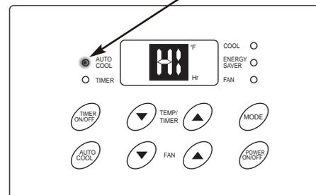
Note: Fan starts at High Speed and adjusts to a slower speed as the room temperature dictates. For example if the room doesn't get too warm, it will stay at the slowest speed. If the room temperature rises quickly, such as a door being opened, it will automatically go to the highest speed. The fan speeds will re-adjust back to the slowest speed as the room returns to the original set temperature. Press either the fan slower (▼) or fan faster button (▲) to adjust the fan speed manually.
