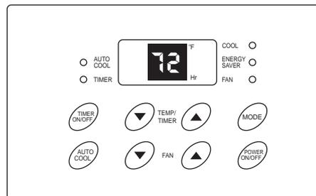
Note: Tap or hold either up (▲) or down (▼) button until the desired temperature is seen on the display. This temperature will be automatically maintained anywhere between 60°F (16°C) and 90°F (32°C). If you want the display to read the actual room temperature See "To Operate on Fan" section.
