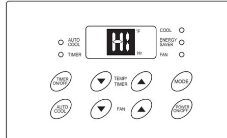
Press the Fan Faster button (▲) will increase the fan speed from Low (LO), to Medium (ME), to High (HI). The digital display will indicate your chosen speed. Press the Fan Slower button (▼) will decrease the fan speed from High (HI), to Medium (ME), to Low (LO). The digital display will indicate your chosen speed. After 5 seconds the display will revert back to the set temperature.
