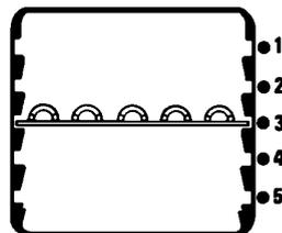
To put the shelf into a different position, keep the front edge raised, slot the shelf on to the runner, lower the front edge and slide the shelf in.
