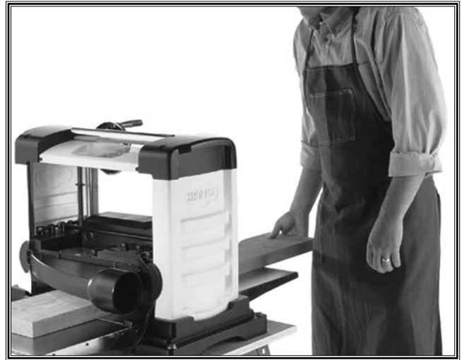
Figure 31. Notice that operator is feeding workpiece from the infeed side and has his body positioned to the side of the travel path.
