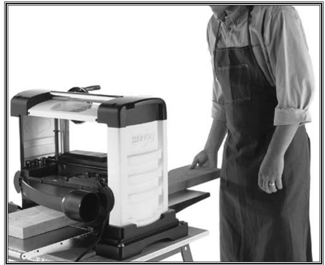
Figure 4. Stand out of the way of the workpiece line of travel.
