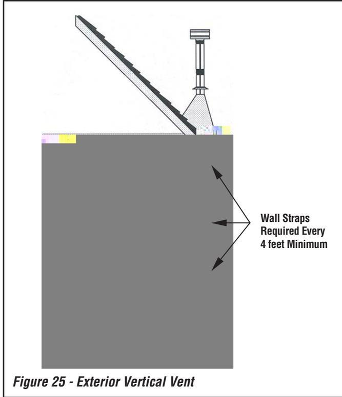
**Preferred Installation – Vertical Vent Through the Roof**
