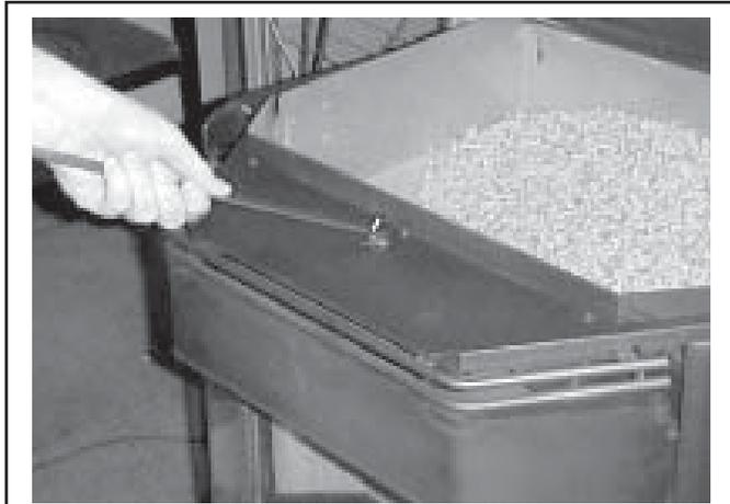
**Figure 37 - Tube Scraper Rod**
