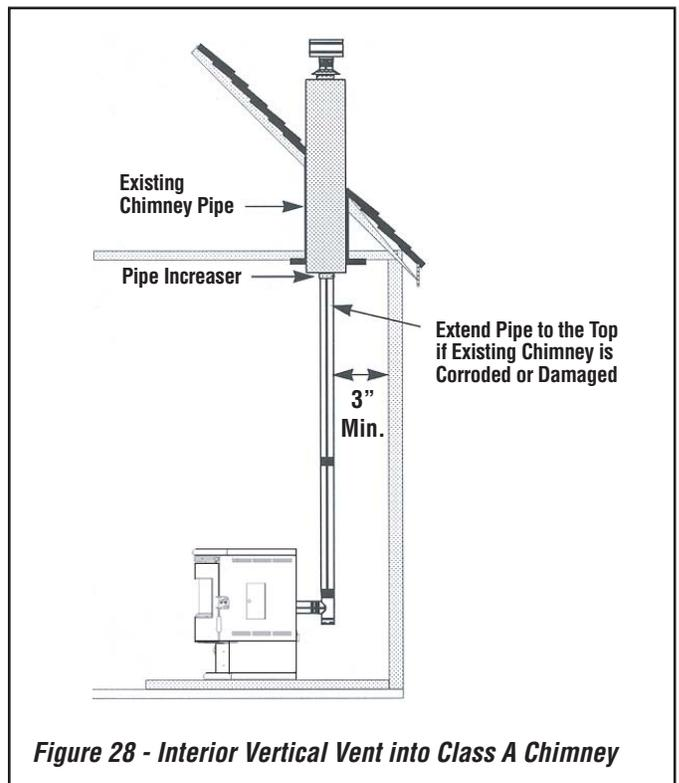
**Standard Installation Configurations Into an Existing Fireplace**
