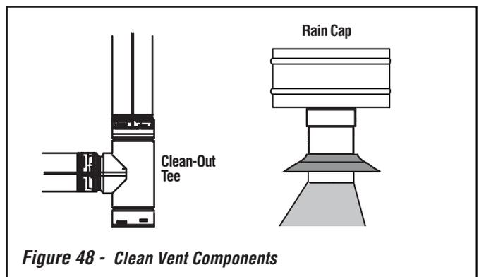
**Figure 48 - Clean Vent Components**
