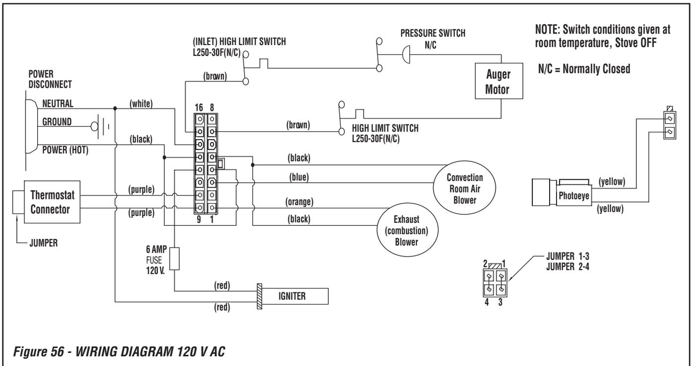
Figure 56 - WIRING DIAGRAM 120 V AC
