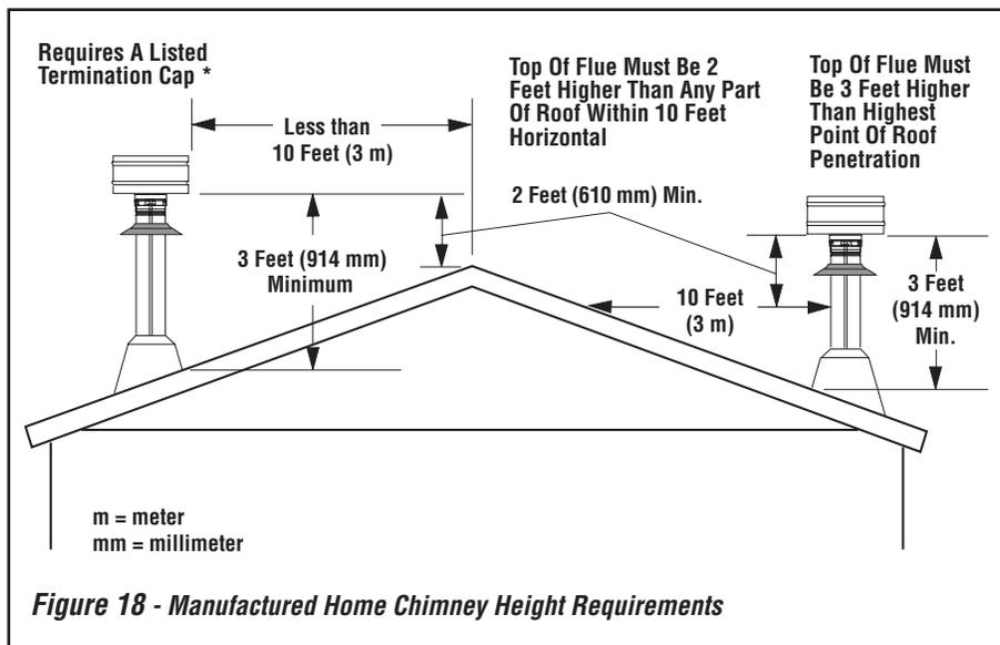
To pass inspection in nearly any jurisdiction, the chimney must meet both safety and exhaust flow requirements. The (3 feet by) 2 feet by 10 feet rule applies to both masonry and factory built chimneys
