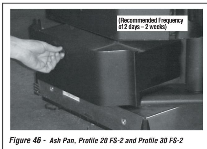
**Figure 46 - Ash Pan, Profile 20 FS-2 and Profile 30 FS-2**
