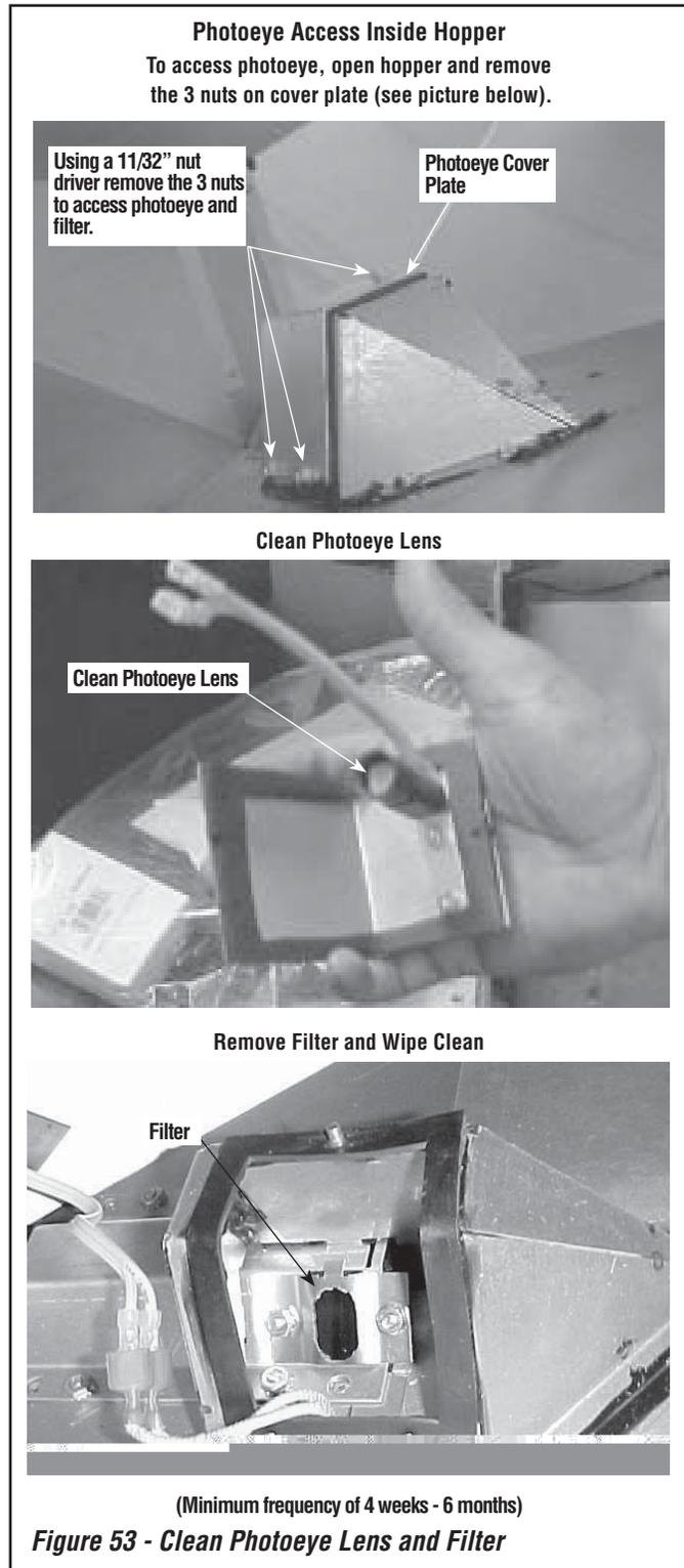
2. Clean Filter as follows: With the photoeye cover plate removed, look inside the opening. You will see an amber colored square glass filter secured in place by a bracket and 2 nuts. Using an 11/32" nut driver, remove the 2 nuts and lift off the bracket. Using your finger slide filter up and out.
