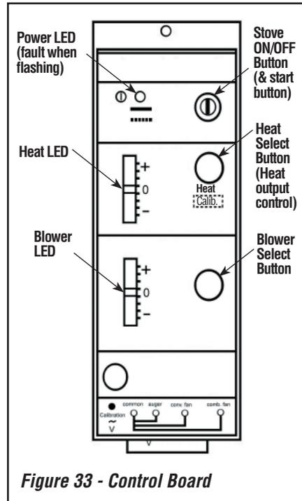
**Note:** The control board has an internal memory which recalls the last setting prior to loss of power. Because we individually check each stove prior to packaging, one of the two scenarios will appear when you first plug in your pellet appliance.
