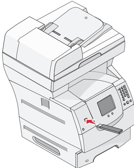
**Note:** If you insert the memory device when the MFP requires attention such as when a paper jam has occurred, the MFP ignores the memory device.
