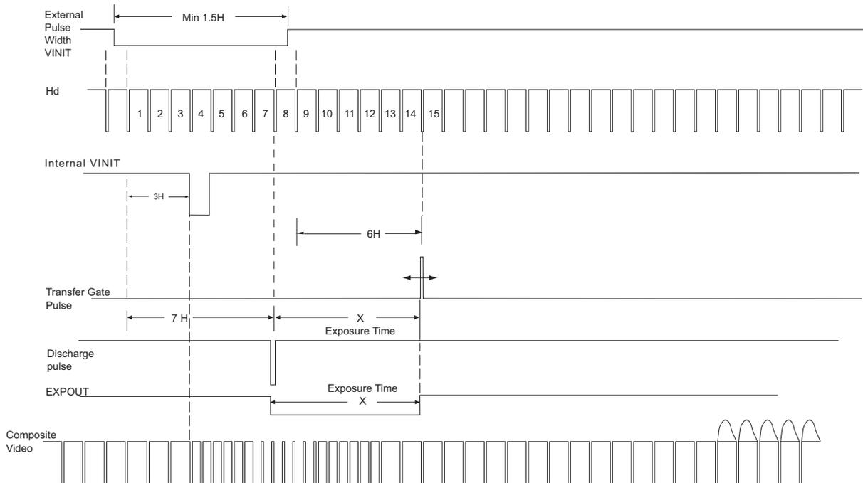
For the progressive format, one frame of video output will start from the rising edge of the pulse width control. At async mode with external pulse input high, the video output will be disabled as the camera continues discharging the CCD image, providing black video only.
