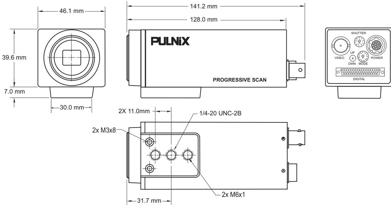
FIGURE 16. TM-6710CL Physical Dimensions
