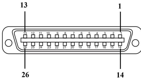
FIGURE 5. MDR 26-Pin Connector (0226-622VC)
