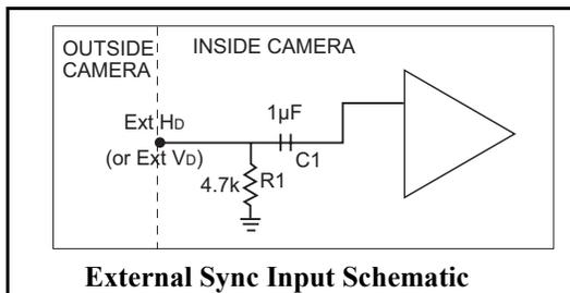
The internal sync generator will take external VD to generate internal VD. External VD frequency should be the same as the frame rate.
