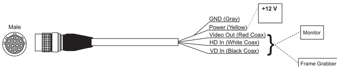
**Note:** Make sure that the unused leads are not touching and that there is no possibility that the leads could short due to exposed wires.
