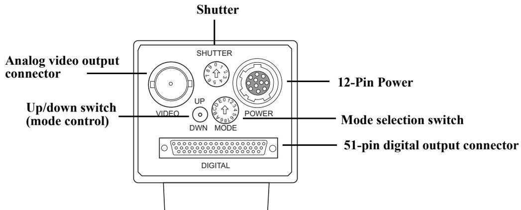
FIGURE 9. Rear Panel Layout (TM-6710CL)
