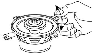
Figure 3. Mounting the GTO6425 or, not shown, the GTO7525.
