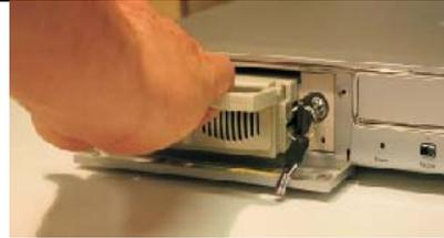
Carefully lift the handle on the front of the caddy and remove it from the housing.
