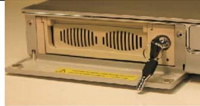
Open the cover of the hard disk enclosure and unlock it using the supplied key. When unlocked the key will be vertical as shown.
