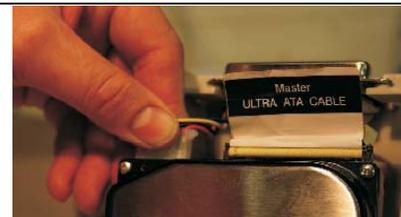
Connect the power connector to the power socket on your hard drive. The connector fits with the cut off corners at the top.
