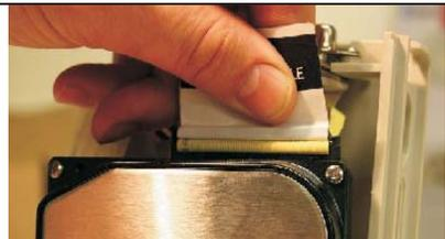
Place your hard drive in the caddy and then connect the data cable to the socket on your hard drive.
