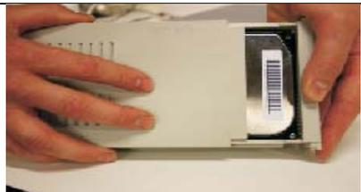
Slide the top cover of the caddy towards the end with the handle to replace it.
