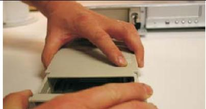
Slide the top cover of the caddy towards the back (the end with the connector) and remove it.
