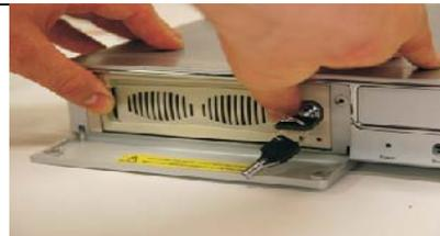
Replace the caddy into the housing pushing on both sides to ensure a solid connection, then turn the key to the horizontal position to lock it.
