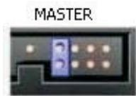
Prepare your hard drive by setting the jumper to Master. Check the label of the hard drive for information on how to do this.
