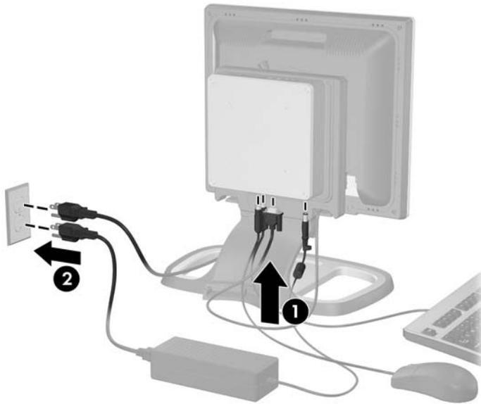
6. Slide the power supply tray out from the base of the stand (1) and place the Thin Client power supply into the tray (2). Route any loose cables through the cables guides on the sides of the tray (3).
