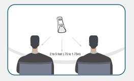
With the microphone in position, un-mute the microphone by pressing and releasing the MUTE button (confirm by viewing flashing GREEN LED).
