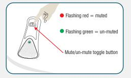
To turn microphones off, first mute the microphone, and then plug it into the Charger Base. Make sure the RED LED turns on.
